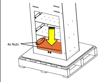
Re-install the lower Internal Shelf onto the 4x thread studs of the Pedestal & install the 4x Nuts.
