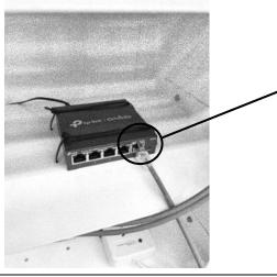
Connect the Ethernet Cable from the base of the Pedestal Loom into the TP-Link Ethernet Router.
