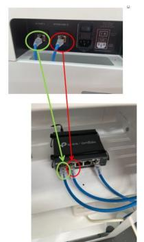
Connect the 2x Ethernet Cables from the Kiosk Rear Cable Entry Ports into the TP-Link Ethernet Router as highlighted.
