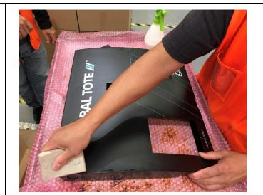
Once Decal is located correctly, squeeze the water trapped between the Decal & Top Door Assy using a Soft Felt Squidgy.
