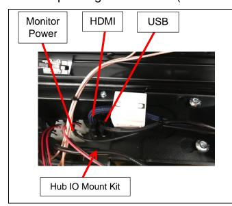
Connect 3x LCD Screen Loom plugs into the Hub IO Mount Kit.
