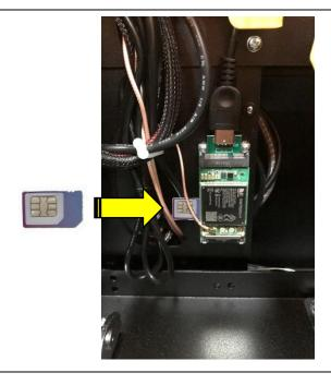
Insert SIM Card into Modem from the rear in the orientation shown.
