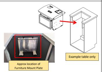
As required, remove the old machine from the fixed table – check that the Furniture Mount Plate is not damaged.
