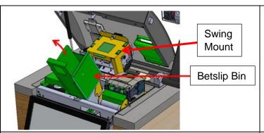
The Modem is in the Main Frame against the rear wall, behind the Betslip Reader Swing Mount.
