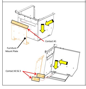
Ensure that the TSST Kiosk is located into the Furniture Mount Plate using the 3x points of contact in areas shown.
