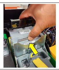
Push the locking rod in the direction shown on the BNA to disengage the BNA Head from the rest of the mechanism.
