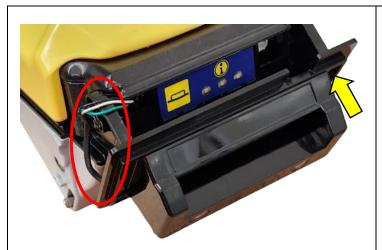
Reassemble the LED Bezel onto the BNA Head.
