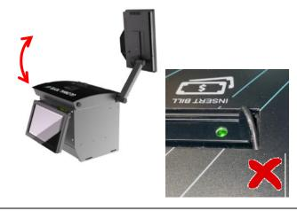
Open & close TSST Lid whilst watching the NFC Cable, to ensure that it does not route towards the Bezel Beak.
