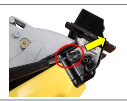
Pry the LED Bezel from the BNA Head using a small screwdriver (or similar) to disassemble it.
