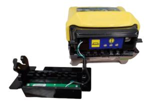
Once disassembled, separate the LED Bezel from the BNA Head.
