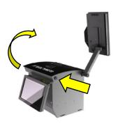
Unlock and open the Top Door by pushing the Button on the RH side of the Top Door.
