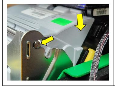
Re-install the BNA Head back into the mechanism and push it downwards.
