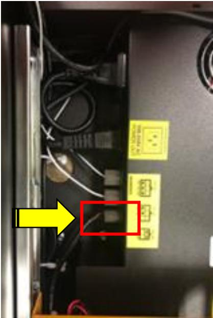
A photograph showing the interior of a power tray. A power connector is being inserted into a port on the left-hand side. A red rectangular box highlights the port area, and a yellow arrow points to it.            | Reinstall the 1x Power Connector into the LH Side of the Power Tray. |
